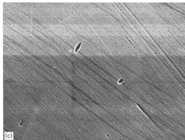
Figure 2 Scanning electron micrograph after the breakdown of the passive film for (a) 316 SS, (b) alloy 926, and (c) alloy 31, in the simulated FGD environment.
